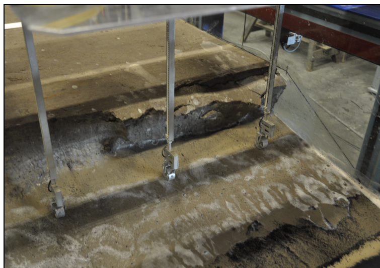
Figure 2.3 Profile followers of the wheel profiler used to measure the cross-shore dune profile
