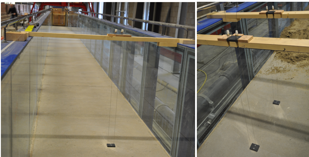
Figure 2.4 Layer thickness meters mounted on the concrete lower part of the dune profile
