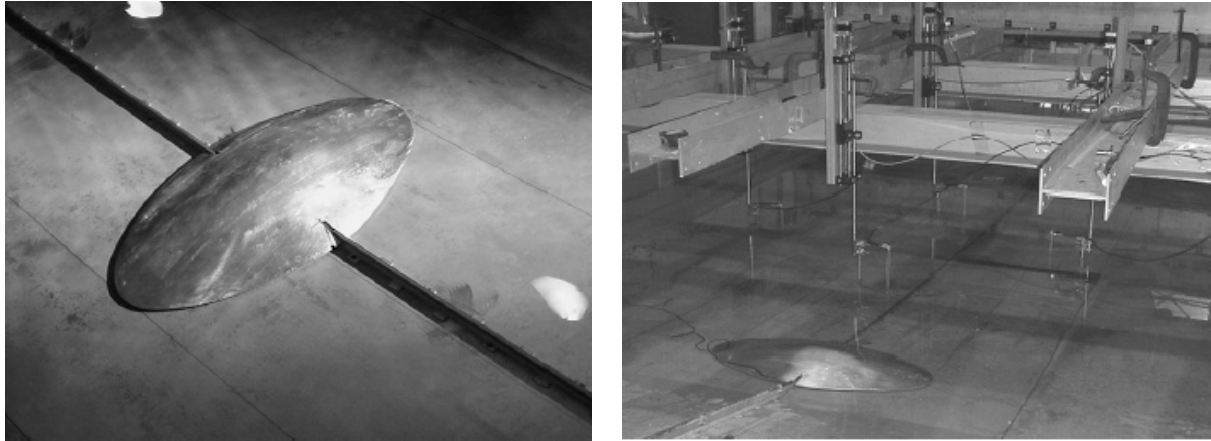
Figure 3.15. Photographs from the 3-dimensional tests of Enet et al (2003). The photo on the left shows the flattened dome-like model landslide mounted to a guiding rail. The photo on the right shows the array of capacitance wave gauges, used to measure wave heights, placed over the wave tank.
