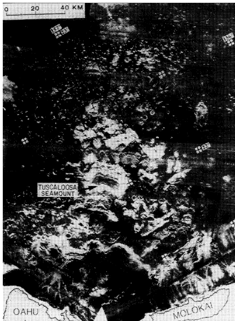
Figure 2.9. Side-scan sonar image of the Nuuanu (off Ohau) and Wailau (off Molokai) debris avalanches, Hawaii. Individual displaced blocks, the largest being the Tuscaloosa Seamount, appear as distinct light areas, generally becoming smaller away from the islands (Hampton et al. 1996).
