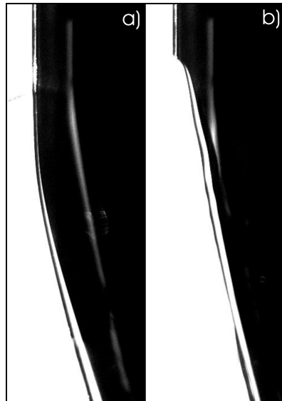
Figure 4.16. Raw images of a) wave run-down, and b) wave run-up, illustrating the issue of meniscus reversal. Image a) shows the draw-down of the shoreline as the landslide initially accelerates down the slope. Image b) shows the wave run-up that occurs moments later. Note that the 15° sloping beach is shown as vertical in these images.
