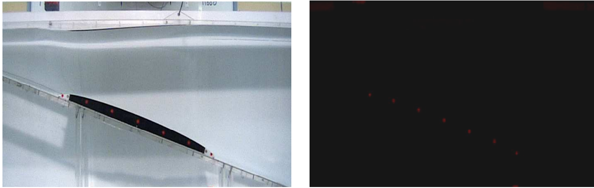
Figure 4.5. An original image (left) and its processed image (right) to remove all but the red dots on the side of the sliding block prior to the PTV analysis to find the landslide's kinematics.
