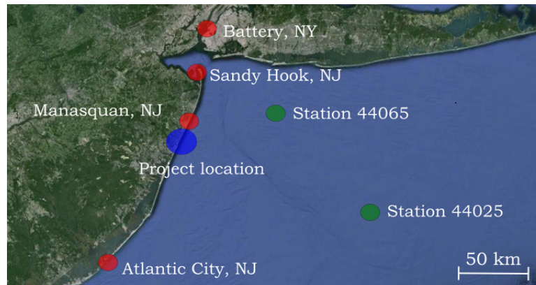
Figure 4.5 Location of information sources used for determining the accuracy of two other models to apply at the boundaries of XBeach (nesting). Red are tidal gauges, green are wave buoys and blue is the project location. [Source: Google Earth].
