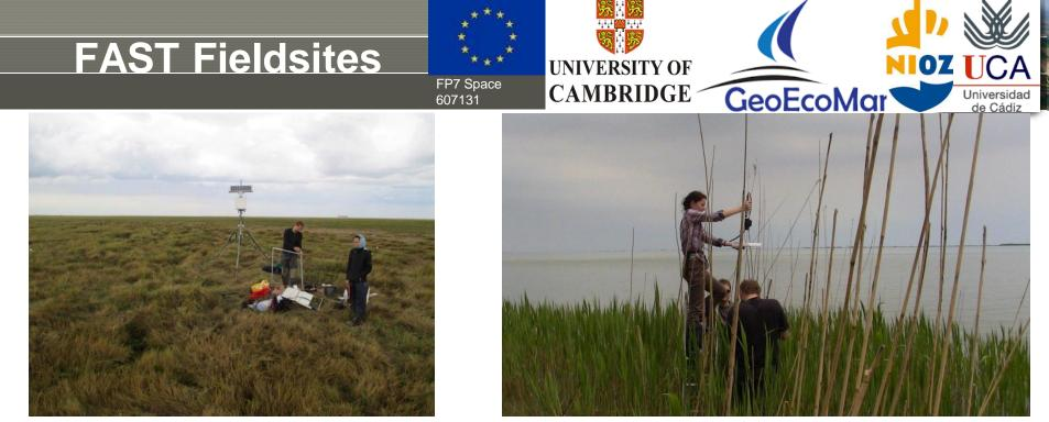
Measurements of in-situ spectra and vegetation dimensions at Romanian field site to link spectral EO data to local vegetation properties.
