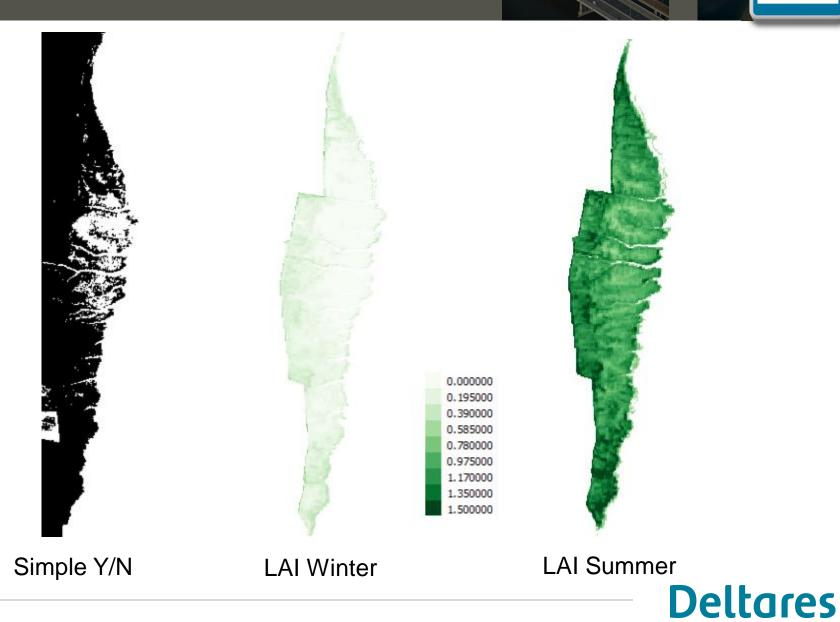
LAI  $[m^2/m^2] = N \times b \times h_v [m^{-2} \times m \times m] = vegfactor in Xbeach$
