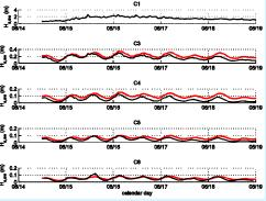
rapid swell wave height decay from C1 to C3 and swell variance on reef well predicted. small phase delay due to bottom friction.
