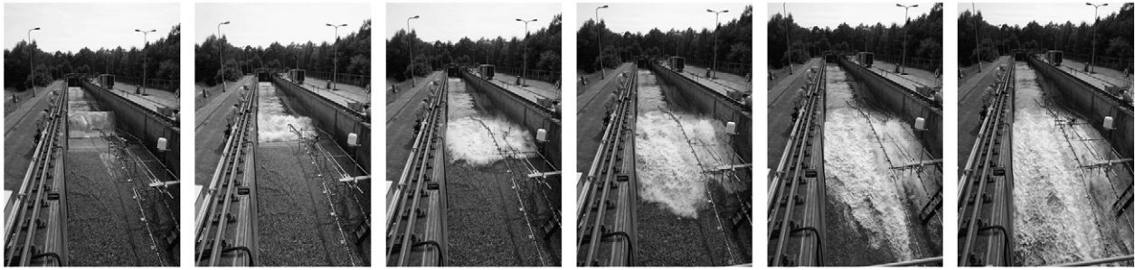
Fig. 8. Typical barrier overwash sequence during simulations of storm conditions and high tidal levels.
