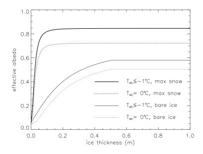
Figure 4: Albedo as a function of ice thickness and temperature, for the two extrema in snow depth, for the default (CCSM3) shortwave option. Maximum snow depth is computed based on Archimedes' Principle for the given ice thickness. These curves represent the envelope of possible albedo values.
