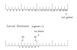
Figure 5: Grid parameters for a sample one-dimensional, 20-cell global domain decomposed into four local subdomains. Each local domain has one ghost cell on each side, and the physical portion of the local domains are labeled ilo:ihi. The parameter nx\_block is the total number of cells in the local domain, including ghost cells, and the same numbering system is applied to each of the four subdomains.
