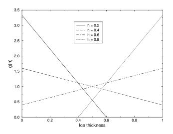
Figure 3: Linear approximation of the thickness distribution function g(h) for an ice category with left boundary  $H_L = 0$ , right boundary  $H_R = 1$ , fractional area  $a_n = 1$ , and mean ice thickness  $h_n = 0.2, 0.4, 0.6, and 0.8$ .
