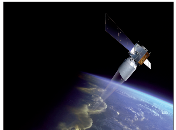
Figure 2. Artist impression of the ESA earth explorer mission ADM-Aeolus that will provide a global coverage of wind information for the first time in history (courtesy ESA).
