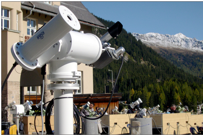
Figure 4. Left panel: KNMI instruments for the measurement of direct solar radiation present during the 10th International Pyrheliometer Comparison, Davos, Switzerland, autumn 2005. Right panel: histogram of the relative difference between the KNMI measurement standard for direct solar radiation (Eppley HF cavity radiometer) and the World Radiometric Reference (WRR).
