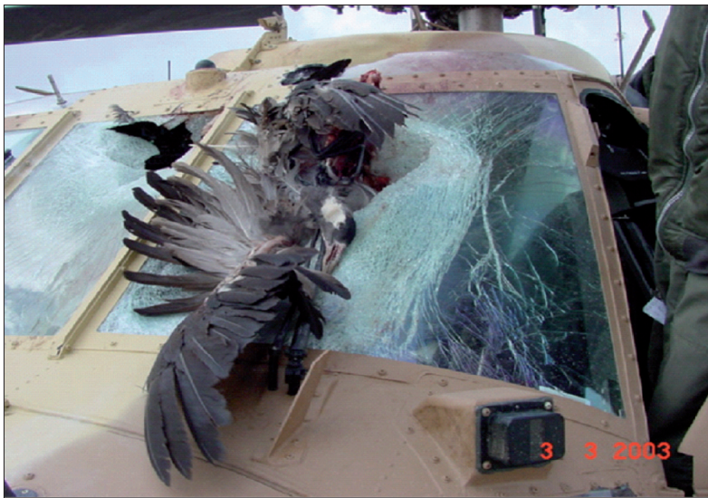
Figure 7. A full hit of a crane on a military helicopter flying at 300 meter altitude in Israel. Cranes migrate in large numbers over Israel in March (photo obtained via RNLAf).
