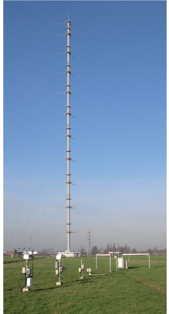
Figure 2. Photographs showing the BSRN station and the 200 m tower in Cabauw. The basic radiation measurements consist of global, direct, diffuse and downward longwave radiation. In addition, various spectral solar radiation measurements are made. Images of the sky are made using a Total Sky Imager. Photographs taken by W.H. Knap, January 2005.
