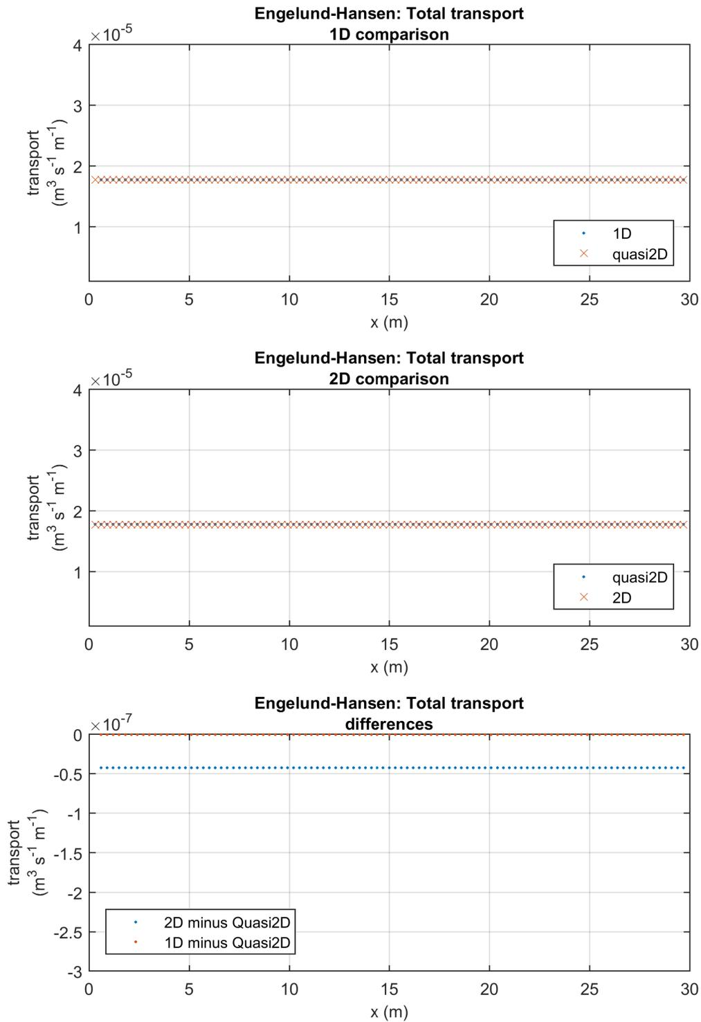
Figure 8: The total sediment transport after 300 min for Scenario 2. The total sediment transport is no longer changing in time.
