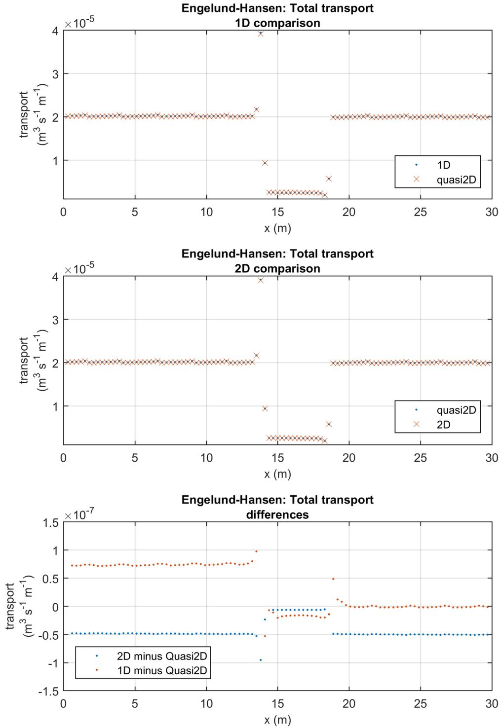
Figure 10: The steady state total sediment transport for Scenario 3.
