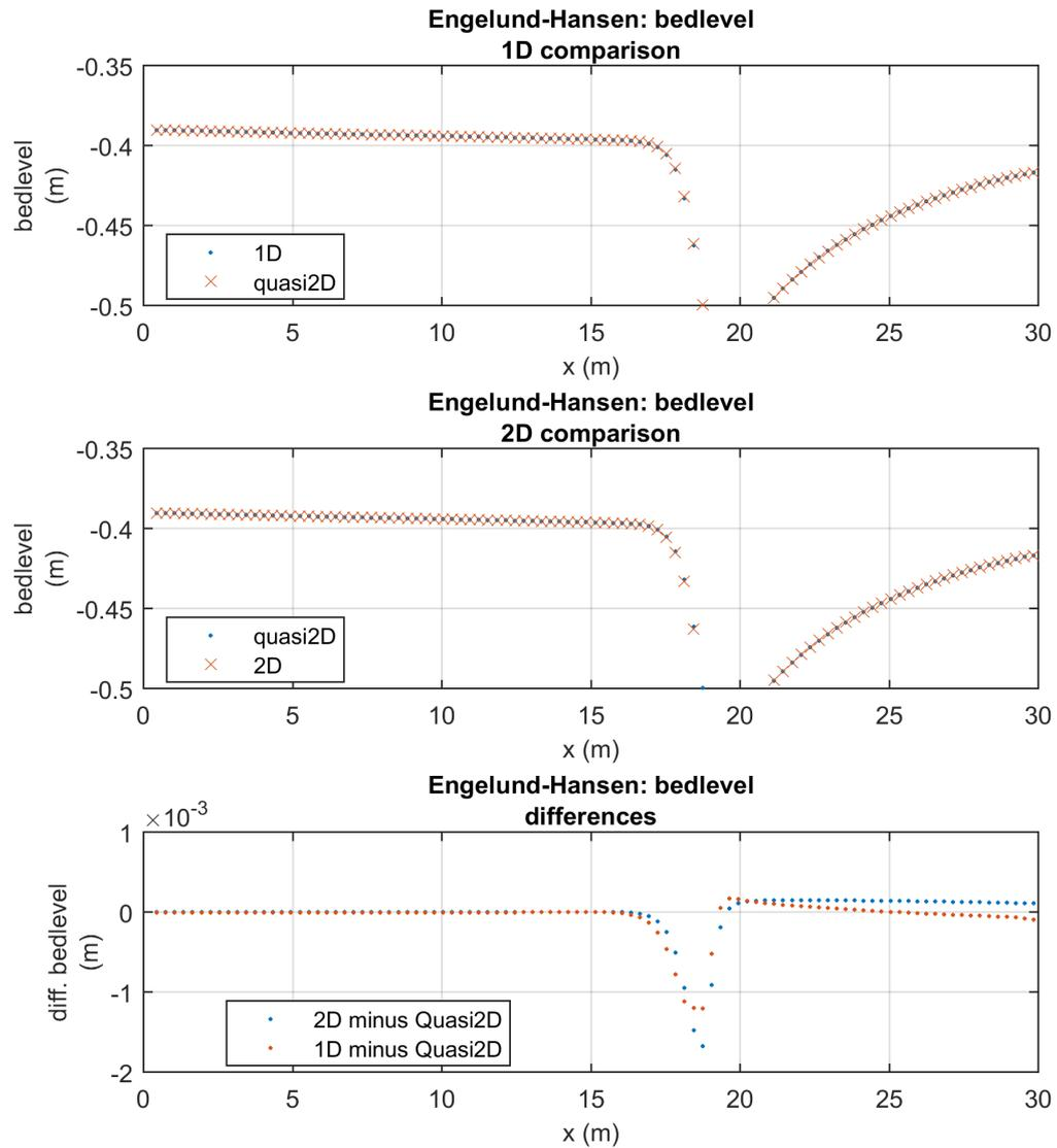
Figure 11: The bathymetry for Scenario 4 after 30 min. The trench is still migrating in the current direction.
