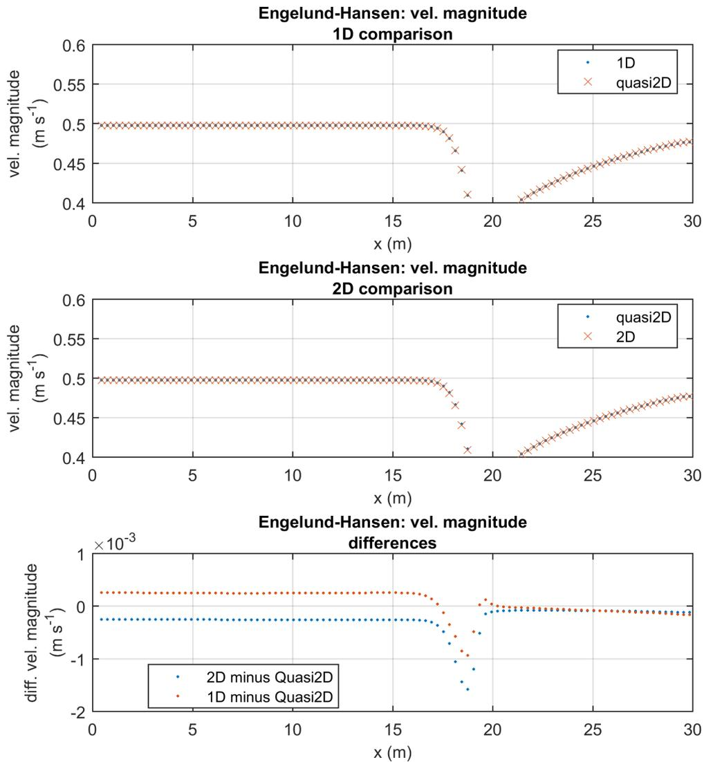
Figure 12: The flow velocity for Scenario 4 after 30 min. The trench is still migrating in the current direction.
