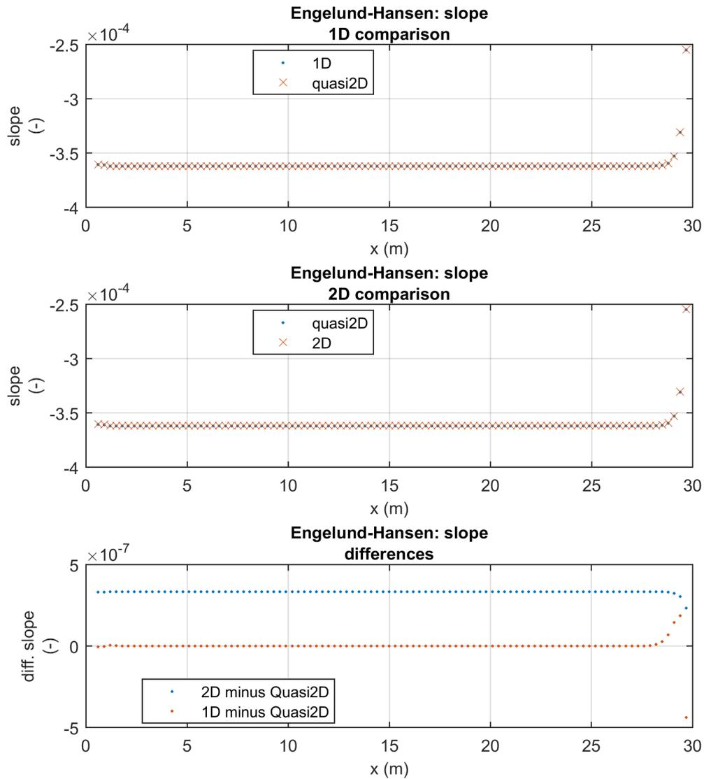
Figure 6: The slope of the bed for Scenario 2 after 300 min. The bathymetry is no longer changing in time.
