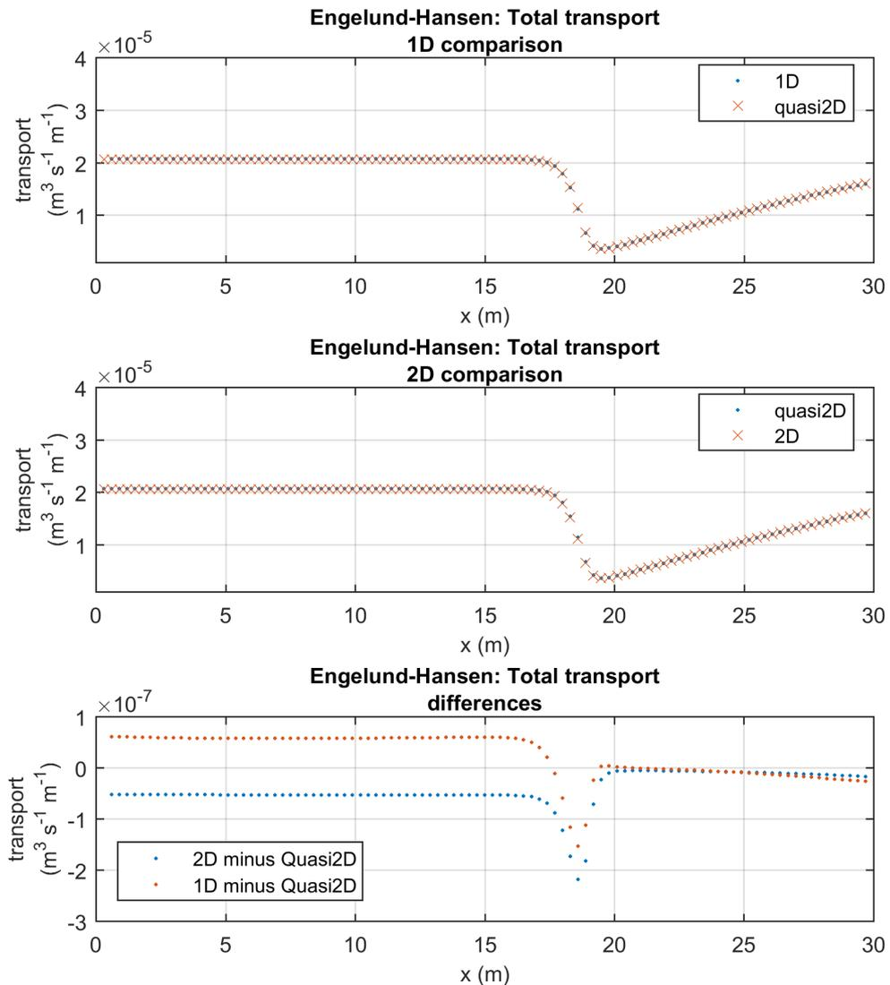
Figure 13: The total sediment transport for Scenario 4 after 30 min. The trench is still migrating in the current direction.
