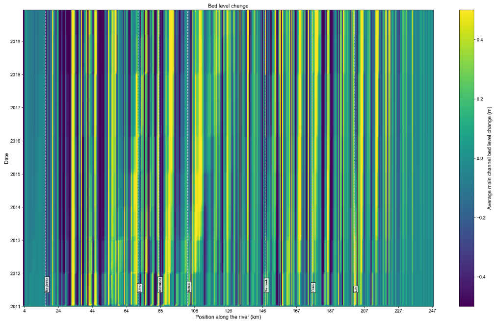
Figure F. 18 Validation j11 – Temporal and spatial main channel averaged bed level change. The colour depicts the change in bed level.
