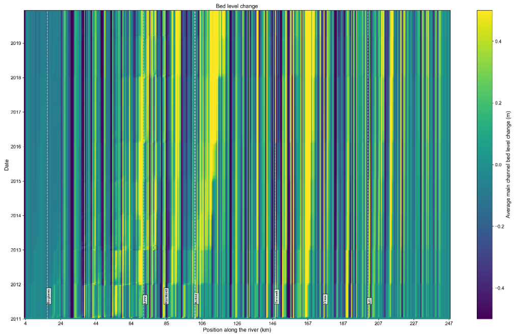
Figure F. 23 Validation j19 – Temporal and spatial main channel averaged bed level change. The colour depicts the change in bed level.
