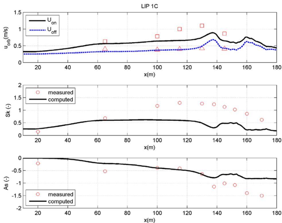
Figure 4.10 The on- and offshore orbital velocities, velocity and acceleration skewness of the LIP-1C case.
