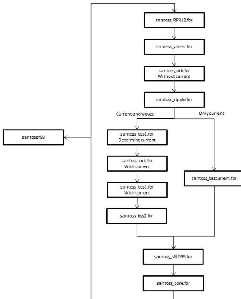
Figure C.1 The relation between the SANTOSS codes in Delft3D.
