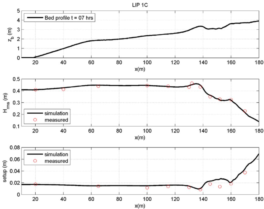
Figure 4.7 Bottom profile, water level setup and representative wave height of the LIP-1C calibration case at 7 hours.
