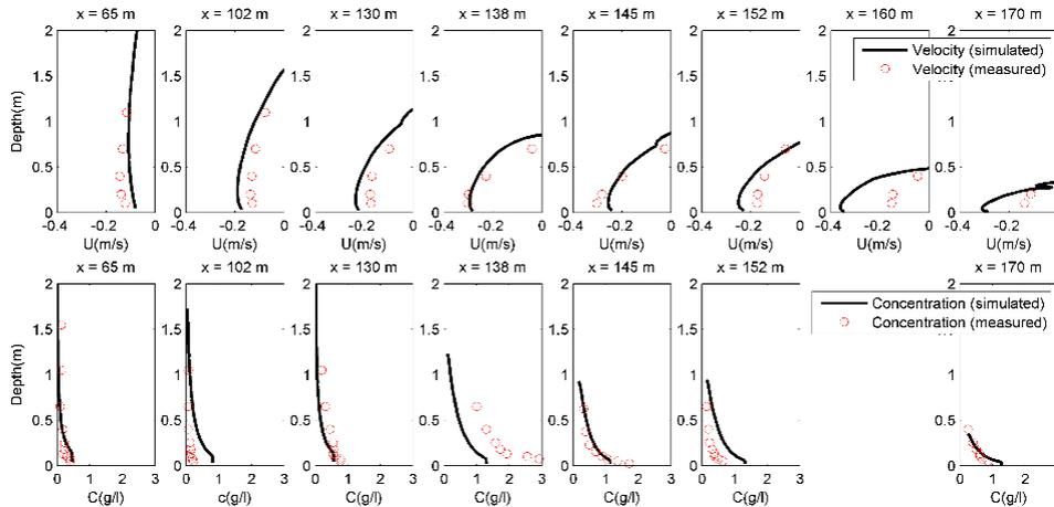
Figure 4.6 Velocity and concentration profiles along the flume of the LIP-1B calibration case at 8 hours.
