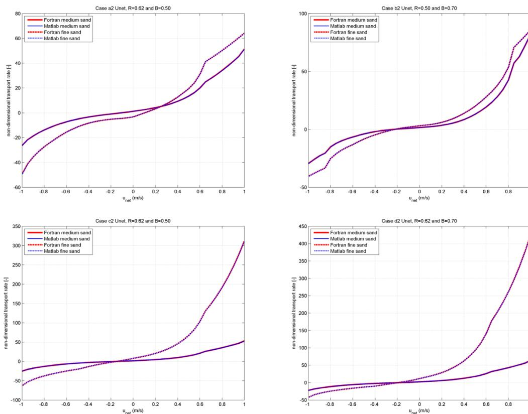
Figure 3.3 Calculation of non-dimensional transport as a function of current ( $U_{net}$ ) for fine and medium sand. For all calculations the wave period  $T=6.5s$ , the water depth  $h=3.5m$ , the root mean square of the orbital velocity  $U_{rms}=0.65 m/s$  and in cases c1-d2 there are progressing surface wave effects.
