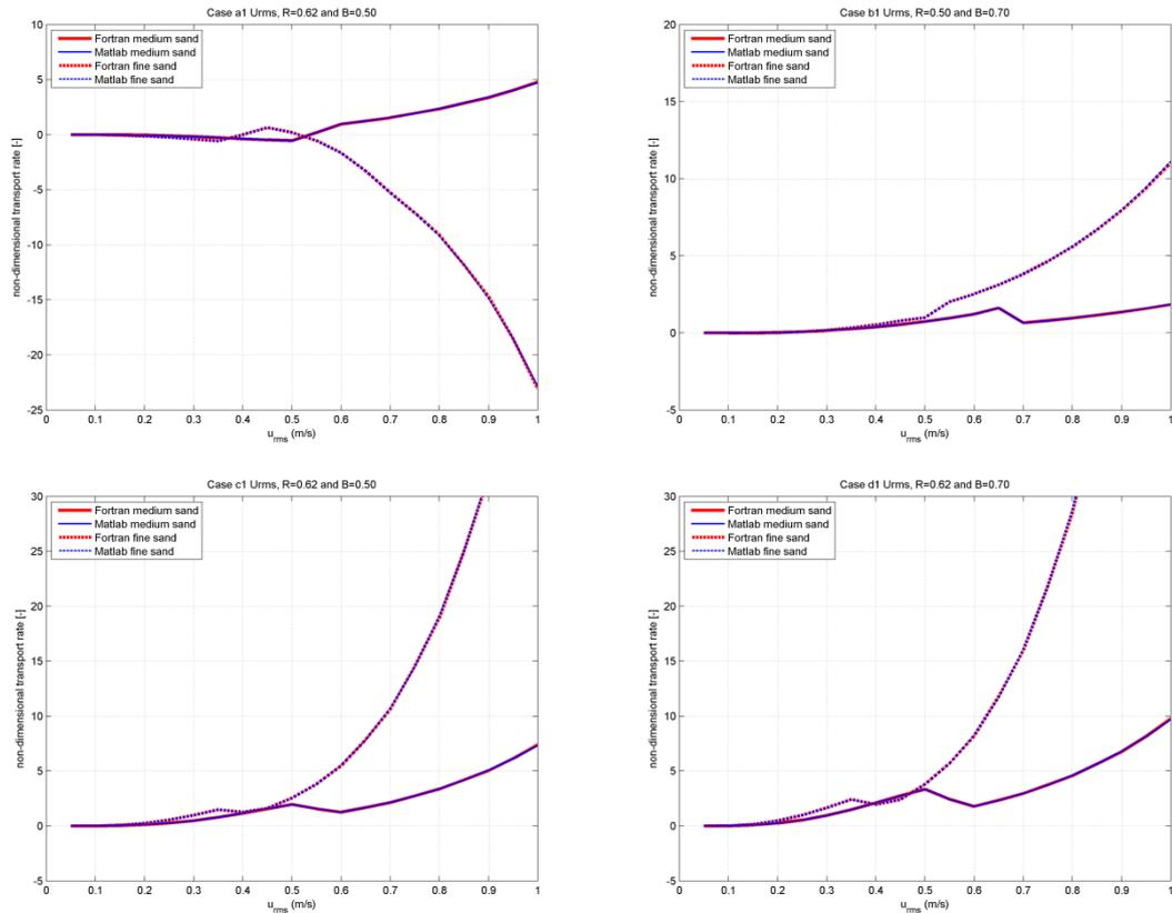
Figure 3.2 Calculation of non-dimensional transport as a function of root mean square orbital velocity ( $U_{rms}$ ) for fine and medium sand. For all calculations the wave period  $T=6.5s$  and the water depth  $h=3.5m$  and in cases c1-d2 there are progressing surface wave effects.
