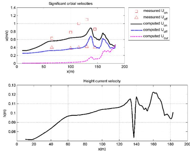
Figure D.6 The top figure shows the magnitude of the modelled orbital velocities with the black (crest) and blue (trough) lines, the magnitude of the measured orbital velocities are the red boxes for the crest and the triangles for the trough. The purple line represents the magnitude of the current velocity at the top of the wave boundary layer which height is presented in the bottom figure. (LIP-1B case).
