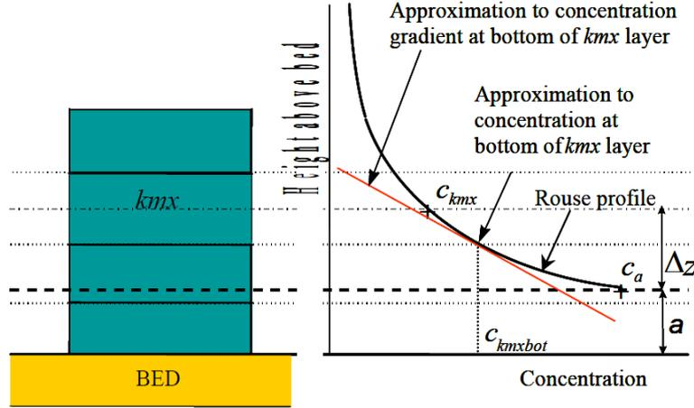
Figure 2.7 Approximation of concentration and concentration gradient at bottom of  $k_{mx}$  layer (Deltares, 2012).
