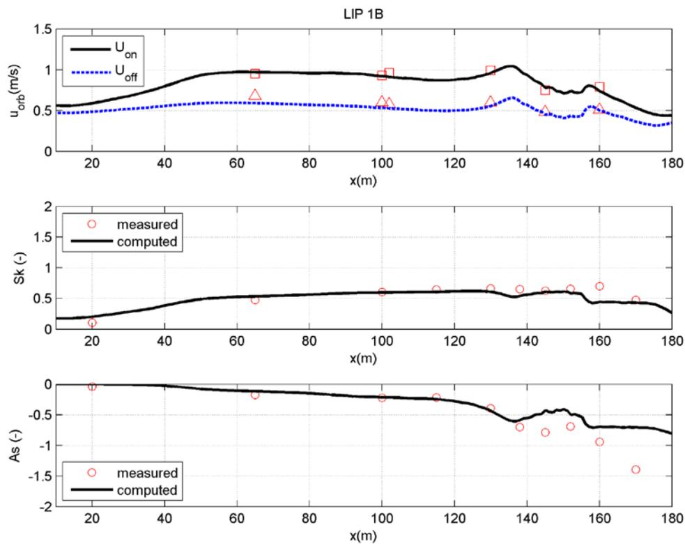
Figure 4.9 The on- and offshore orbital velocities, velocity and acceleration skewness of the LIP-1B case.
